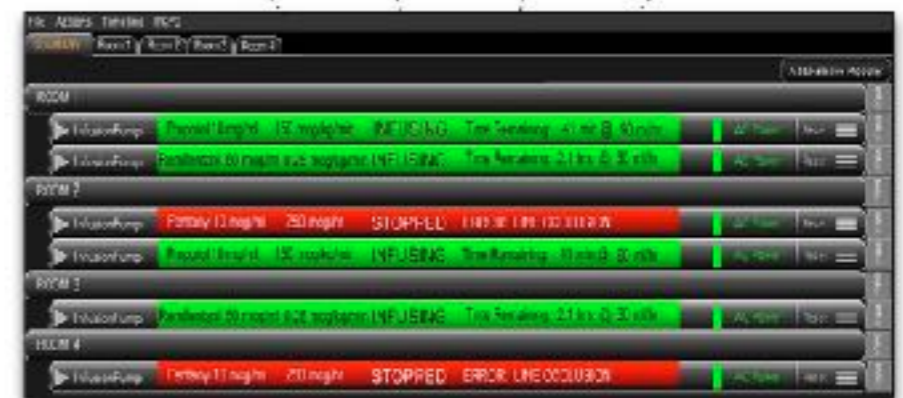
Central Station summary view of all pumps in separate rooms
