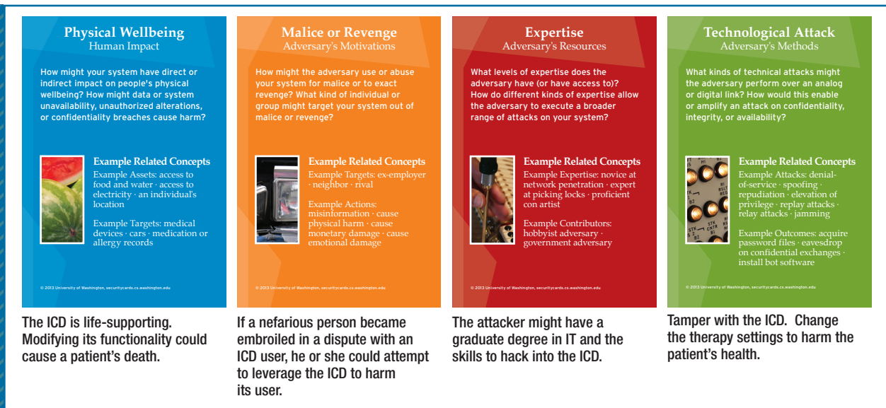
FIGURE 1. Four Security Cards. Developers can use Security Cards to explore potential threats to a technological system—in this case, an implantable cardioverter-defibrillator (ICD).
